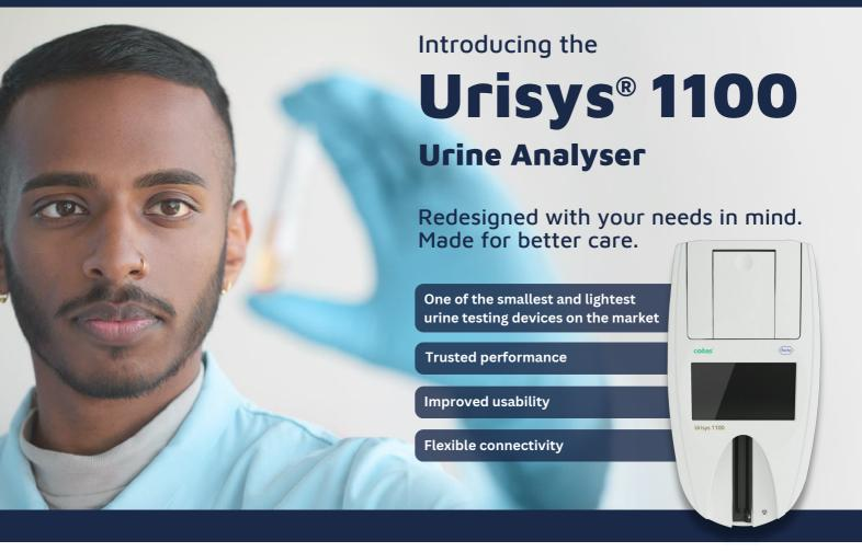
The **Urisys® 1100 system** is a reflectance photometer designed to read and evaluate the urine test strips Combur10 Test®UX from Roche Diagnostics. It reads the strips under standardised conditions, saves the results to memory and outputs them via its own inbuilt printer and/or serial interface. The instrument is intended for near-patient testing.
